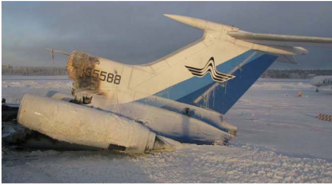
Fig. 9. Tail part of Tu-154B-2 RA-85588 after fire at Surgut airport on January 1, 2011 [2].
