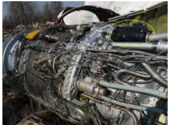
Fig. 14. Generator ГТ40ПЧ6 on Nr 1 (left) Д-30КУ turboprop engine. Photo taken between 11 and 13 April 2010 on the crash site [4].
