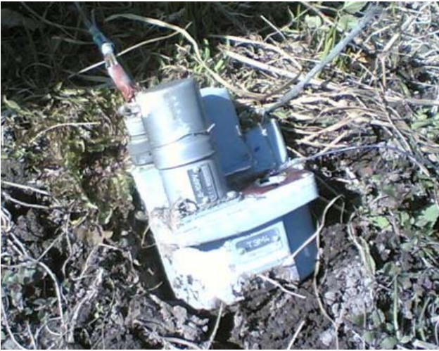
Fig. 15. Electromagnetic brake TЭM-4 for flap control found several meters behind the famous birch tree. Source: http://www.waronline.org
