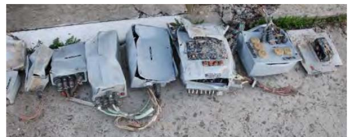
Fig. 13. Junction and control boxes of electrical installation. Photo taken at the site of wreckage storage [4].
