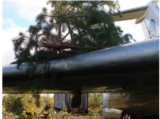
Fig. 11. Emergency landing of Tu-154M RA-85684 at abandoned air strip near town of Izhma on September 7, 2010. The impact was damped by the young trees which have grown since the airport was closed. The photograph shows the right wing that cut a pine tree. http://englishrussia.com/2011/11/04/the-lucky-tu-154/#more-74596
